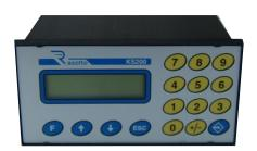
The KS201.1 is a single-quota positioner. The selection of the quota to be reached takes place via the keyboard setting (KEY F). When the start is pressed, the instrument automatically performs the quota by acting on the 4 relay outputs. By moving the axis in manual mode the instrument works as a meter and displays the value supplied by the encoder.
