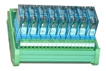
Passive relay interface module that receives digital commands from various electronic devices such as PLCs, industrial PCs, control modules, etc. and controls inductive and resistive loads of small power such as solenoid valves, contactors, small servomotors, lamps, resistors, etc. This type of module has a series of screw terminals that makes it universal and a multi-pin flat connector for quick connection with the whole range of our controllers and instruments.
